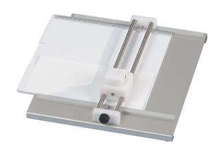
The scoring and cutting of glass TLC/HPTLC plates is a routine in many chromatography laboratories either to economise on plate usage or to cut the plate following separation for further derivatization.
