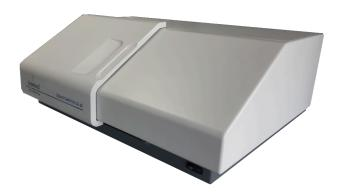
For quantitative determination of samples, the HPTLC-Densitometer CD60 converts the spots/bands of the single substances into a chromatogram curve. It measures the absorbance or fluorescence of separated compounds in transmission or reflection mode. The HPTLC-Densitometer CD60 is controlled by ProQuant software which also enables quantitative evaluation of the generated data.
