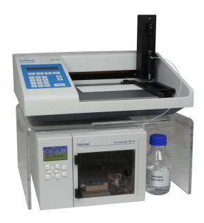
The association of the BS35 auto-sampler with the AS30 HPTLC applicator offers a set of fully automated sample depositions on TLC plates.
