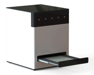
The ProViDoc DD80 is a high-performance documentation system with brilliant recording quality. The workstation consists of a dark hood with different light sources, a camera for taking high-resolution images, a documentation top for guaranteeing the optimal distance between camera and sample as well as a software for controlling the system and saving the recorded images.
